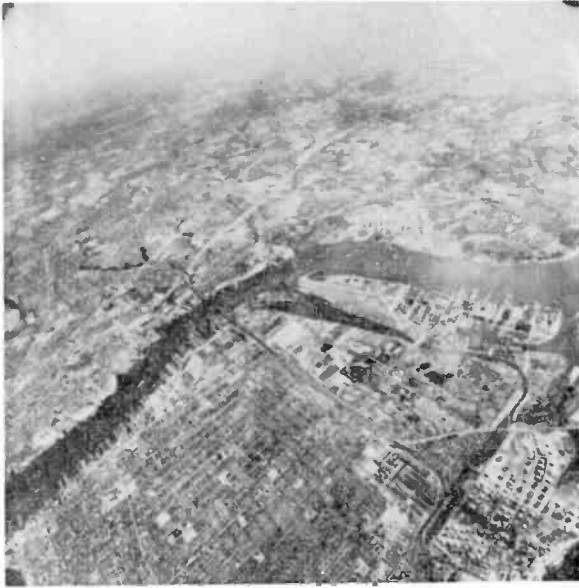
Fig. 45—Photograph of aerial 9-by-9-inch print reproduced on 17-inch monitor picture tube, bandwidth limited to 1800 lines.
